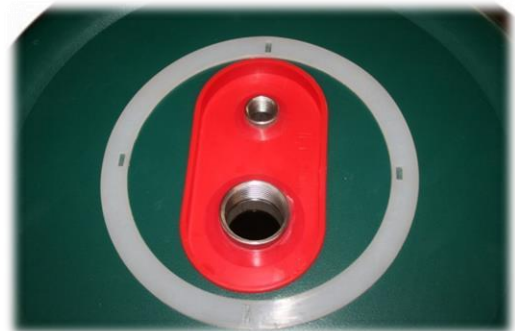
Picture 1.22 Install the backup element and thermostat and the seal for the element cover
