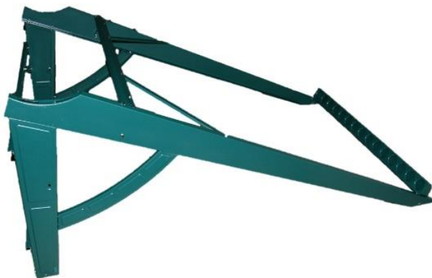
Picture 1.9 Side cross support sections fitted
