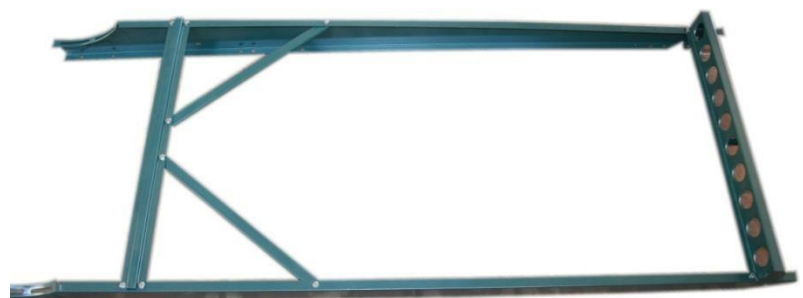
Picture 1.5 Cross support elements added
